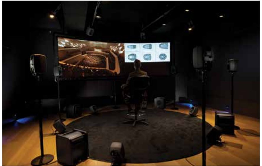
Arup SoundLab – a place to view and listen to buildings, performance environments, and performance sets before they are built physically, or from measurements of real spaces © Andre Costantini
